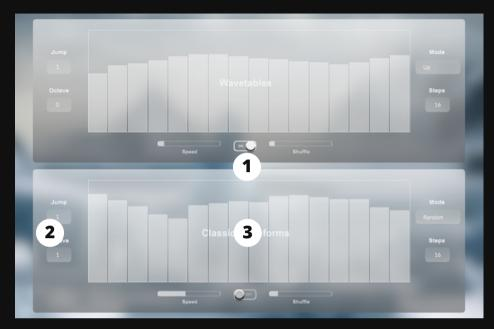
Each layer has an independent arpeggiator that can be turned on or off.
